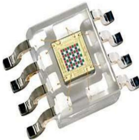
Fig .2. Microscopic view of TCS3200 chip
