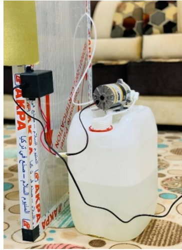
Fig. 3. transformer, pump, hose, and plastic tank contains sterilization solution.
